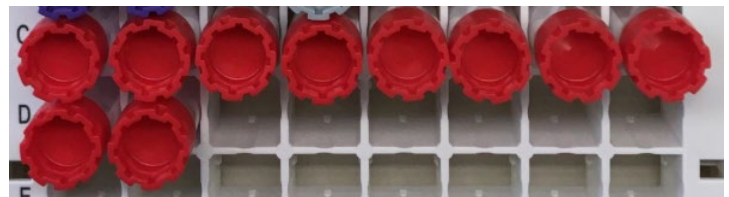
Serum Aliquots: up to 10 (0.5ml each) red cap cryovials possible or nine red capped cryovials (0.5ml) and one blue capped residual (<0.5ml)
